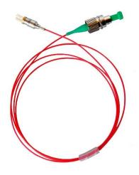
Ortel's 1995 cooled TOSA laser module is characterized for use as a CW coherent optical source laser for LiDAR technology. The 1995 is DC-coupled with a built-in TEC, thermistor, and monitor photodiode. The device is in hermetic TO56 package with 6+1 pins. The 1995 incorporates a high-efficiency coupling scheme to deliver 15 dBm of CW optical power.
